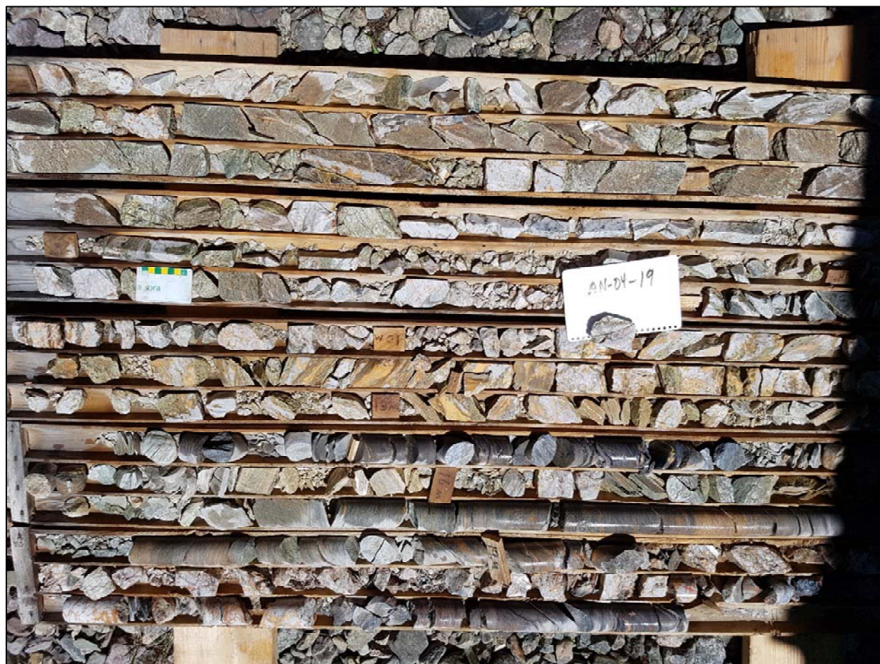
Figure 9-8: Gold Mineralized and Altered Zone in Hole AB-04-19 from the Pit Zone
