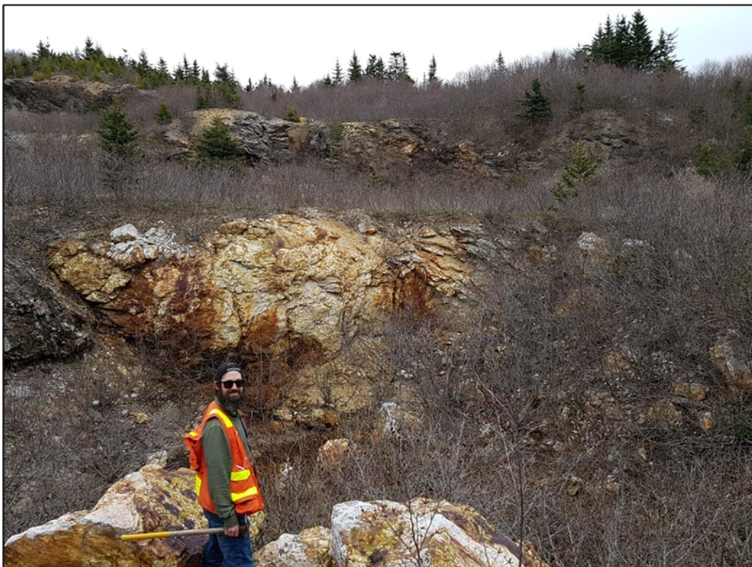
Figure 9-4: Altered and Mineralized Granite Within the Cape Spencer Open Pit. (Note Multiple Rusty Weathering Mineralized Zones on the Far Eastern Wall of the Open Pit)
