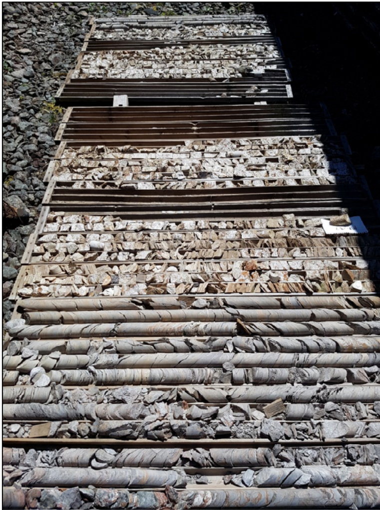
Figure 9-10: Extensive mineralized zone and alteration in hole MR-87 – Road Zone
